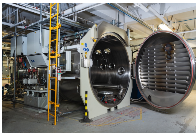
The thermal spray system’s vacuum chamber contains equipment for depositing coatings of reactive feedstock or substrate materials.
