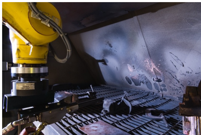
Located at the end of a robotic arm, the cold spray system’s applicator nozzle (shown in the image above at lower left) is used to produce metallic coatings.
